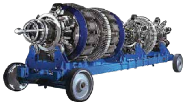
Smart Pig: An internal inspection tool
